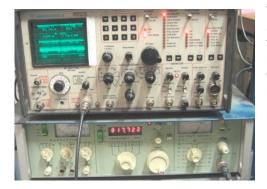
This method is not guaranteed to produce spec sensitivity and squelch operation but will get you in the "ballpark". Using the manual's schematic remember to align the receiver properly once you obtain the proper (compensated) recrystaled channel element for the operating frequency you plan to use. Obviously, for this document is 147.800 MHz.
