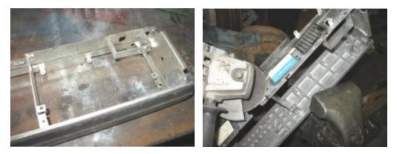
The correct type cage (robbed from an old high-band chassis) was replaced with small bolts and nuts.
